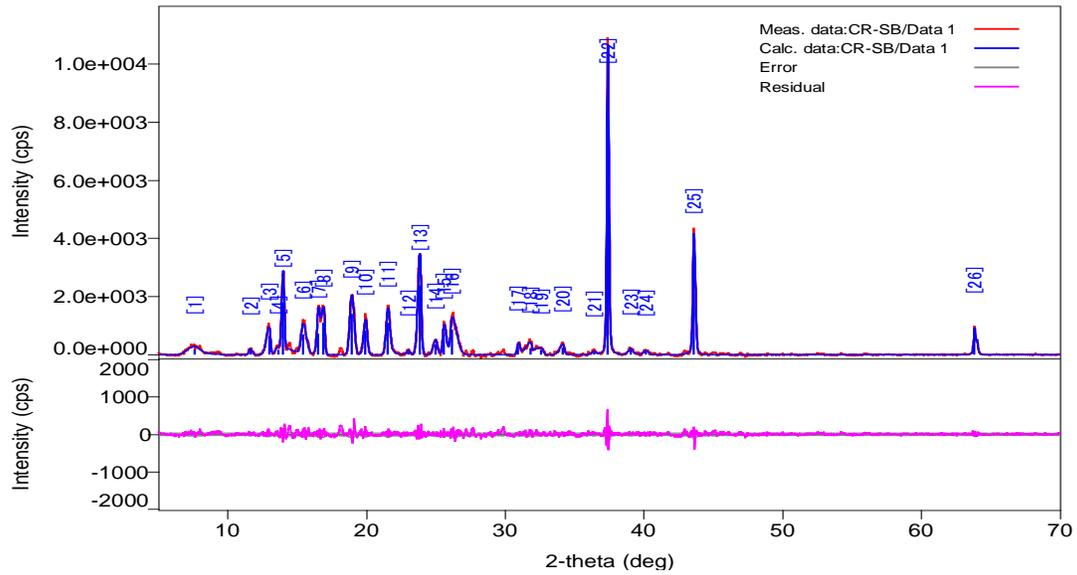
Figure. 2 a) XRD spectrum of SB
