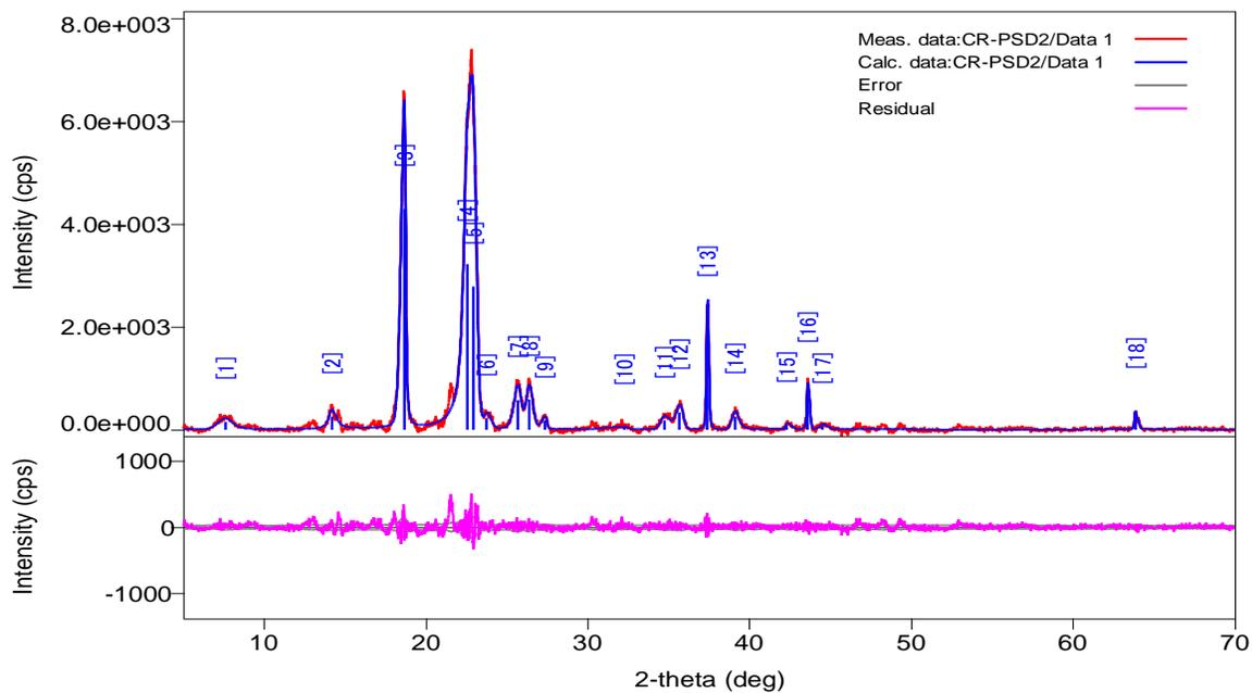
Figure. 2 c) XRD spectrum of SB-PEG complex
