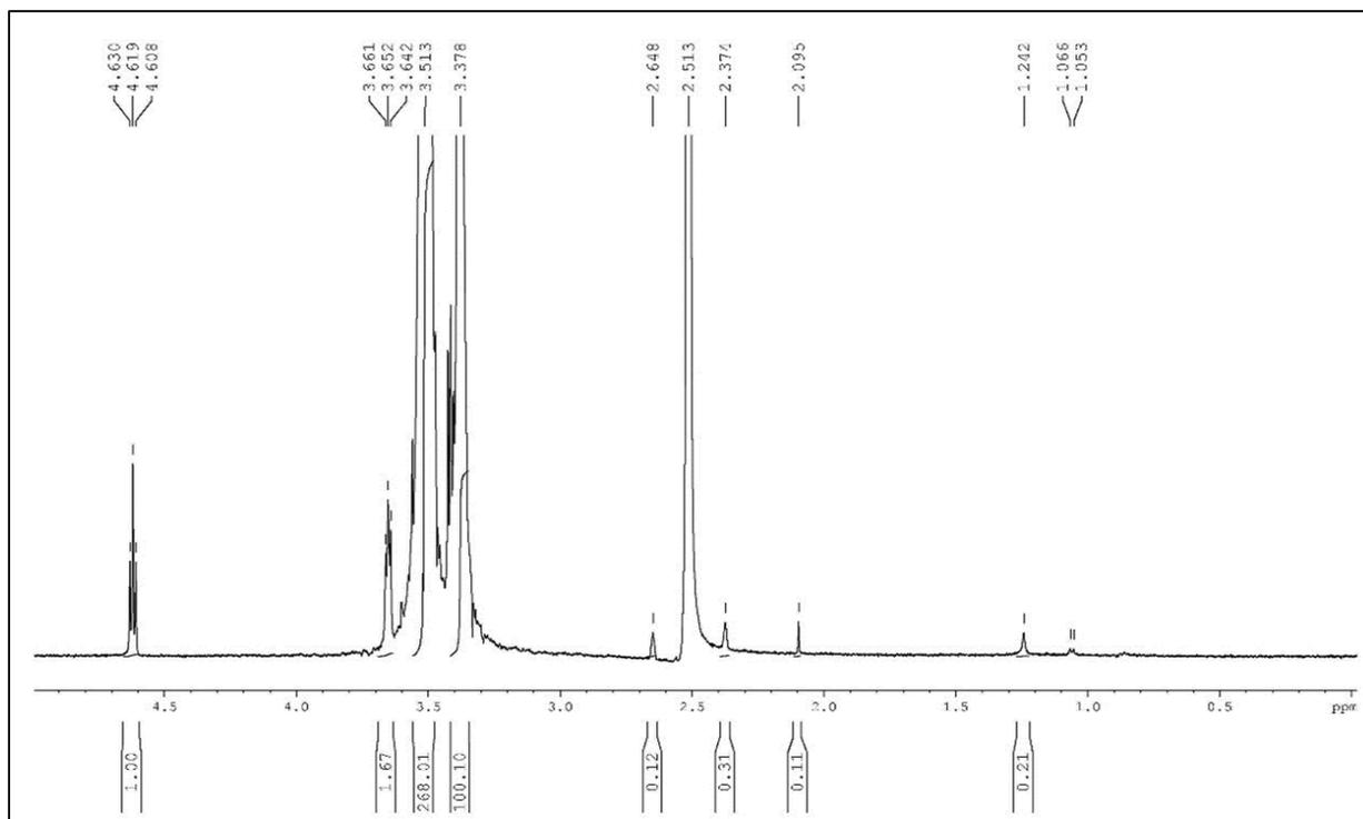
Figure. 3 b)  $^1\text{H}$  NMR spectrum of PEG
